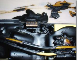
Amps. If allowed to continue in this buzzing mode for more than 60-seconds, the current rises to 4 or 5 amps and within 90-seconds the unit fails from as the resistor/fuse fails. In photo above right, note how the switching transistor has melted the tar around the transistor in less than 90-seconds.
