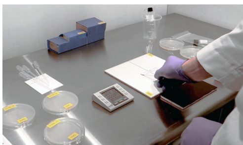
Figure 5: Ceramic tile being dosed with E. Coli and then being treated.
